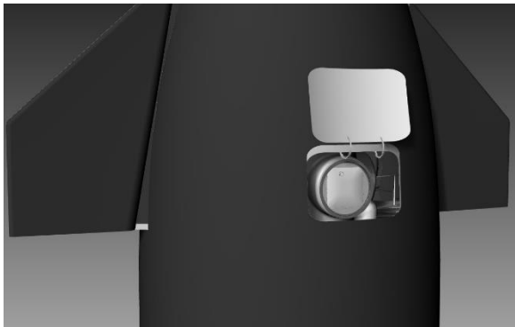
Figure 16. Airlock Outboard Docking Port
